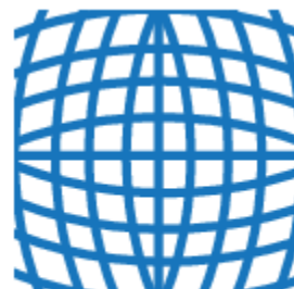
Positive radial distortion "barrel"
